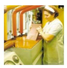
called dressing machine, where the foam is squirted onto the waffles ("dressed"). The next step is to cover the as-yet white whips on the conveyor belt with a high-quality chocolate coating. Temperature plays a major role in this process, as it governs the strength and gloss of the coating. After spending a precisely defined period of time in the cooling channel, the finished whips are then hand-packaged.
