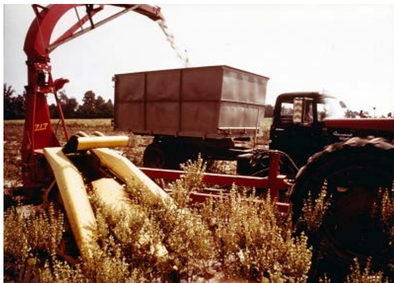
Mechanical Harvesting of Clary Sage into Distillation Bin
