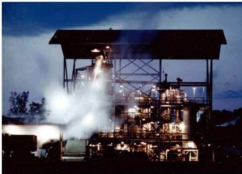
Rotocell in Operation to Extract Sclareol from Plant Material after Distillation
