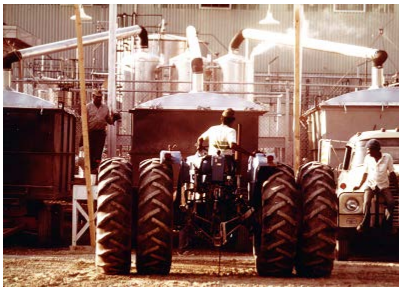
Docking a Truck Bin to the Distillation Unit
