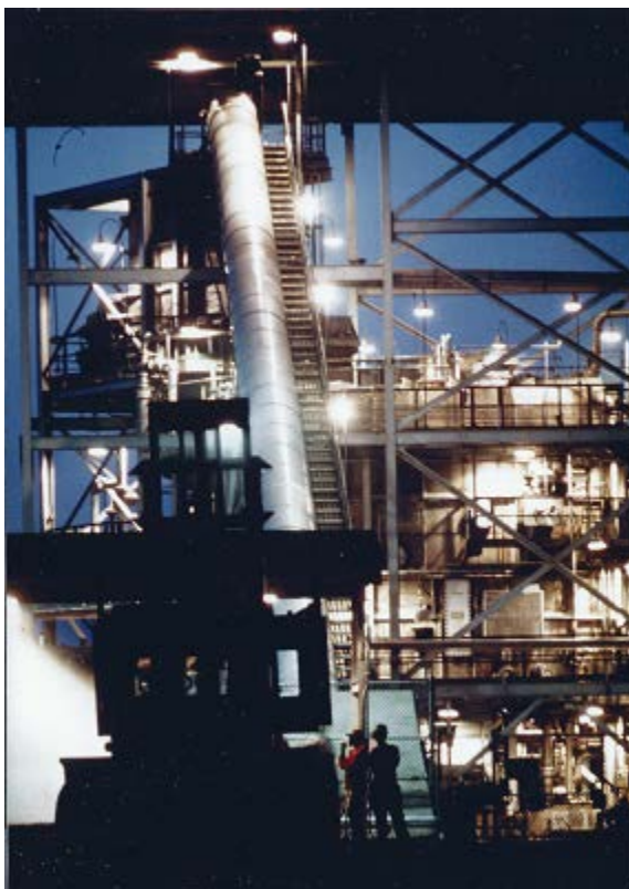
Conveying Plant Material into Rotocell for Extraction
