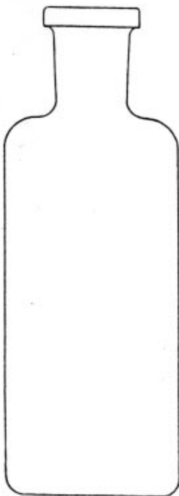
Figure 4 Transfer bottle Capacity 50 to 100 ml
